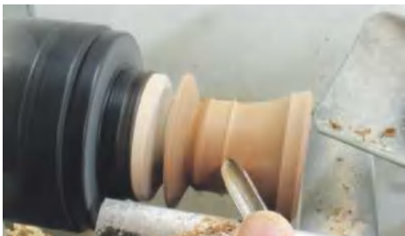
▲ Pic.7 Use a 60 x 60mm piece of sapele, which can be screwed and shaped with a gouge. I decided to go for a Dickensian-style top hat
